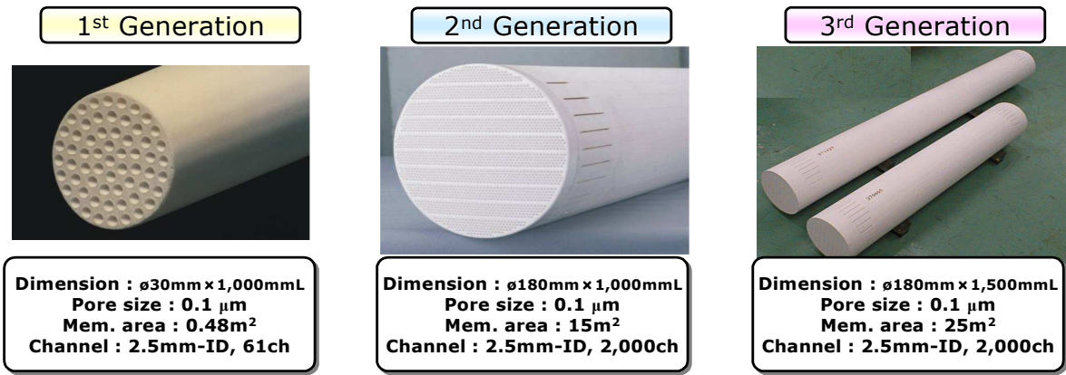
Picture 1. Specification of ceramic membrane
